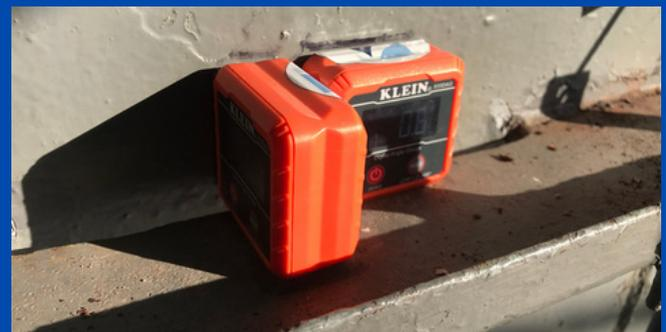
*Digital inclinometers pictured here on The Sullivans. Each of our vessels afloat is similarly equipped with 2 of these devices per ship.*
